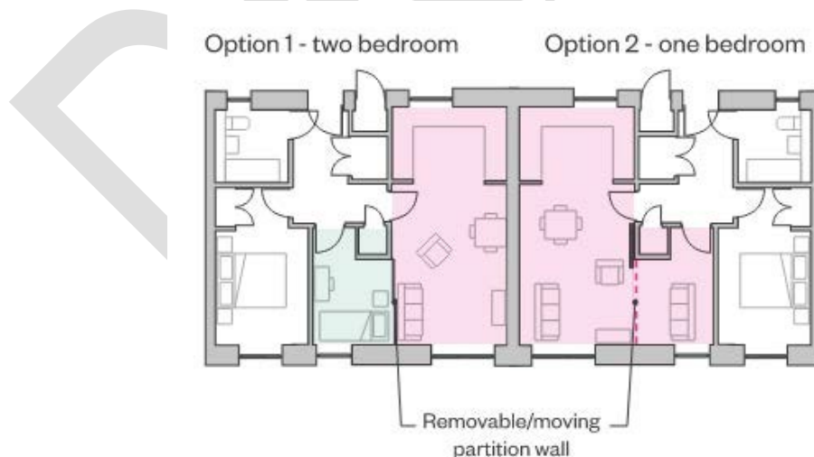
Figure 14: Design for adaptation using a flexible floor plan e.g., one bed flat can be converted to a two-bed flat or a one bed flat with space for home working.
